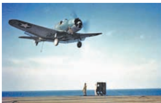
Douglas SBD "Dauntless" scout bomber heads around the deck for a second landing attempt after being "waved off" by the landing signal officer in 1942. Photo courtesy U.S. Naval Historical Center
